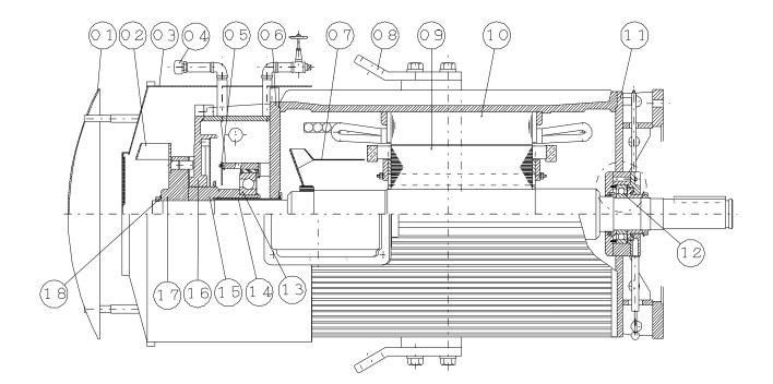
Appendix 4.Typical motor cross sectional drawings : SCIM, TEFC
