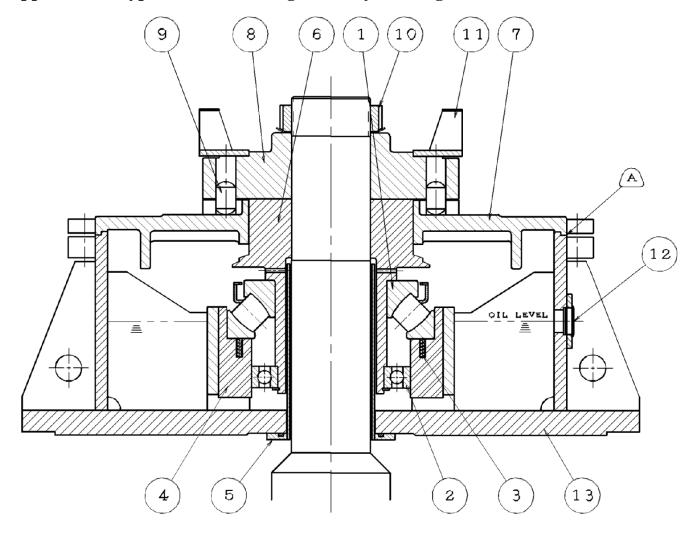
Appendix 10. Typical thrust bearing assembly drawing (vertical machine)
