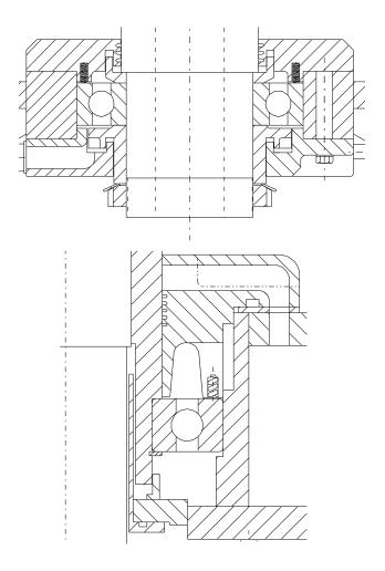
Fig. 4 Upper and lower bearing
