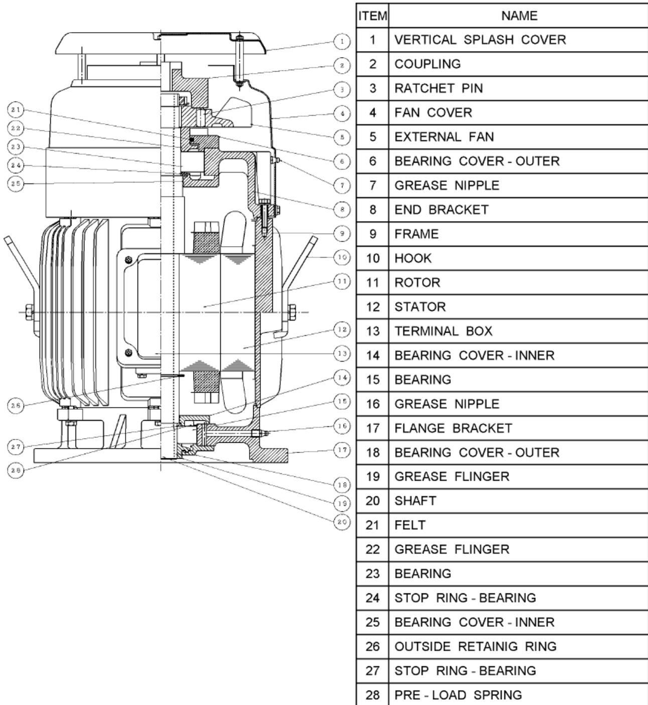
**Appendix 4-2. Typical motor cross sectional drawings : SCIM, TEFC**
