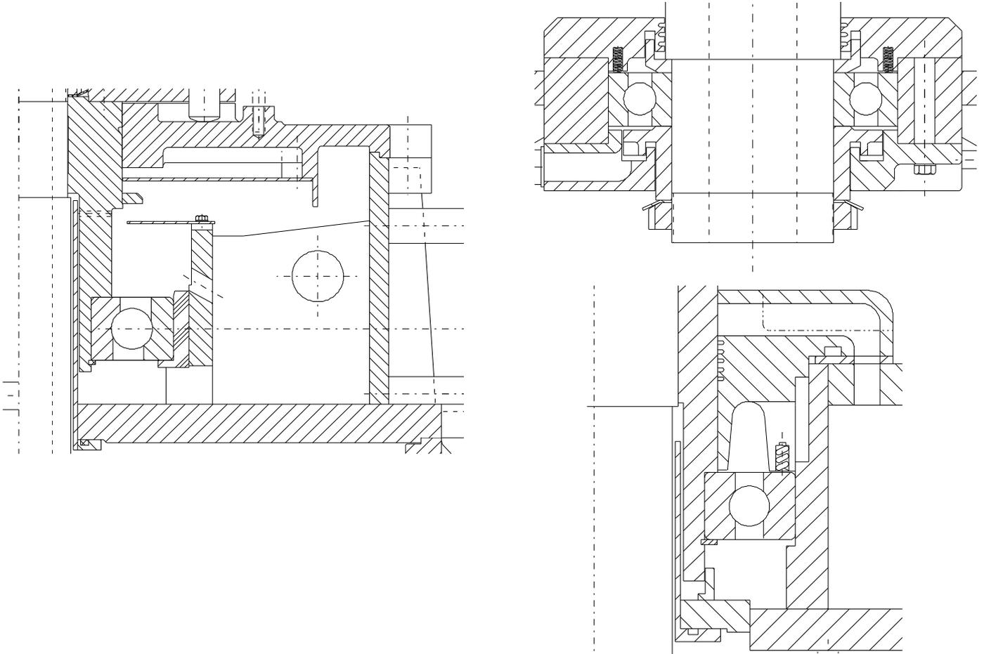
**Fig. 4 Upper and lower bearing**
