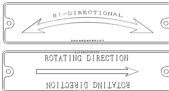
**Fig. 2 Direction nameplate**
