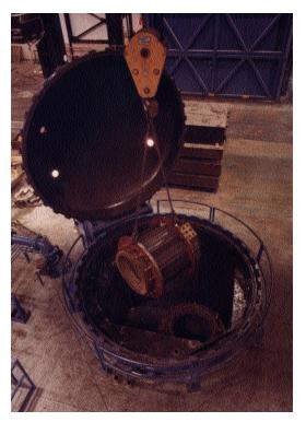
This wound stator is being prepared for vacuum pressure impregnation.
